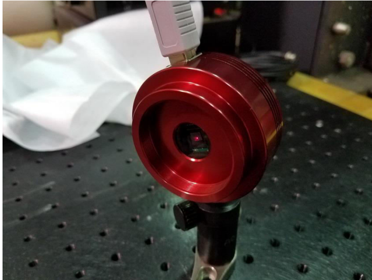
Figure 6 – The science camera is a 1280x960 resolution, 12bit camera. This can be used to measure FWHM values and characterize the system's performance.
